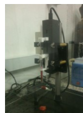
Fig. 2 Electrospinning assembly.
