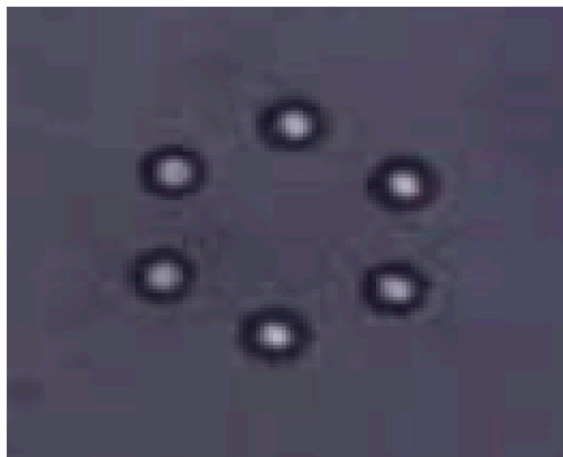
Fig. 1 Six polystyrene beads with a diameter of 3\mu\text{m} being trapped in a hexagonal array. This image was taken in our optical tweezers at Pontificia Universidad Católica.
